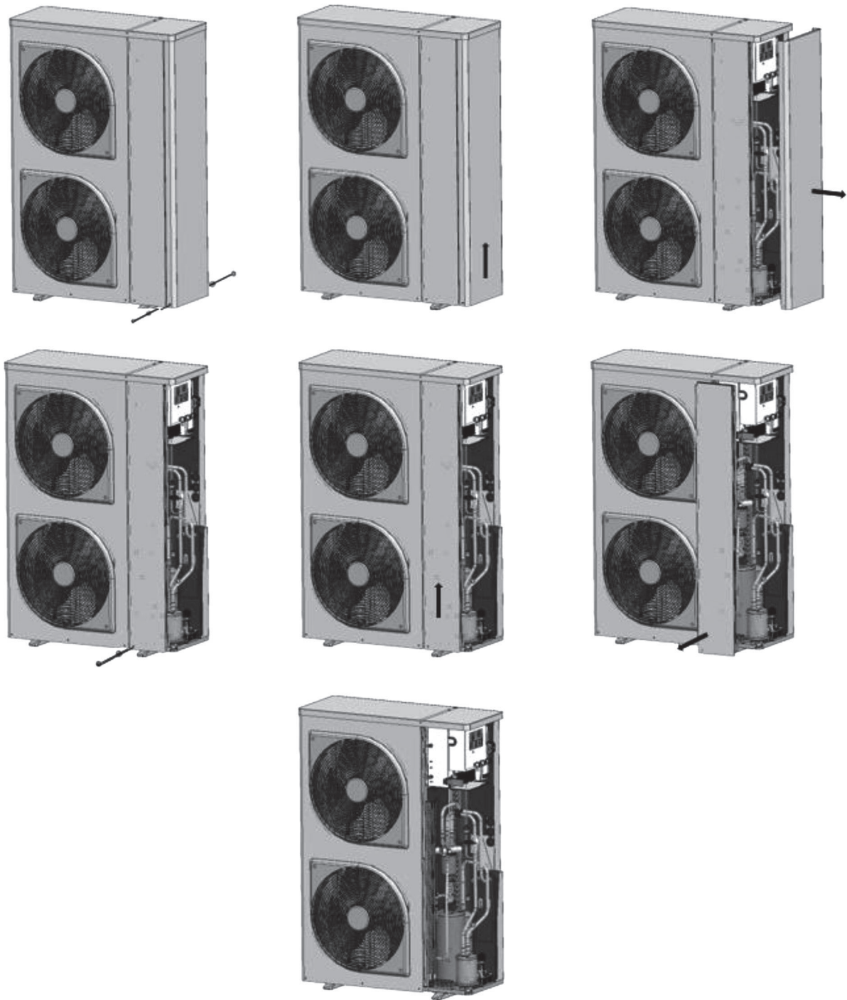
Figure 5 : How to remove front panel for 12 and 14 units
